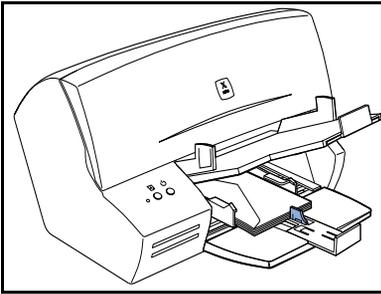
**6** Slide the length guide forward until it touches the bottom edge of the envelopes. Then lower the Auxiliary Tray.
