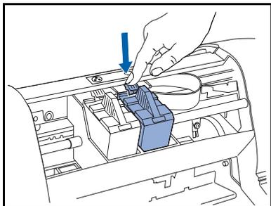
**3** Release the print cartridge by pushing down on the release lever above the cartridge you are removing.
