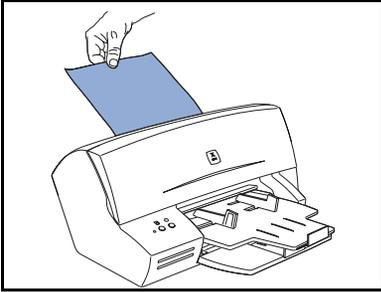
This illustration demonstrates the loading positions for feeding a single sheet into the printer through the Manual Feeder Slot.
