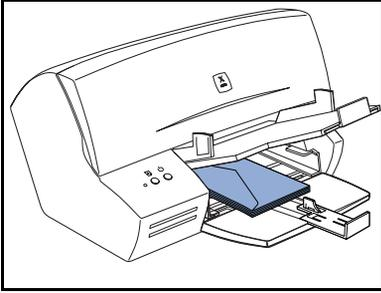
**4** Place a stack of envelopes in the tray. Envelopes must be inserted with their short side as the leading edge, the printing side face down, and the sealing flap on the left.
