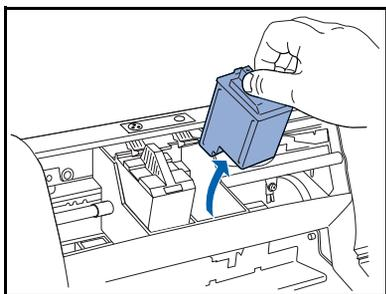
**4** Remove the cartridge by pulling it upwards using your thumb and index finger.
